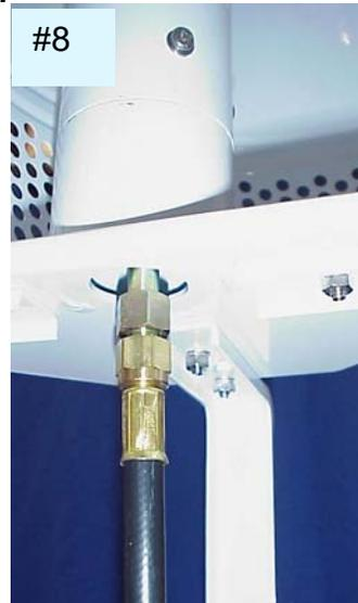
and regulator assembly should go on easily. Hand-tighten the fitting at the hose assembly before using wrenches. Tighten the 3/8" female flare at the end of the hose to the fuel line inlet fitting going through the hole in the base plate with two wrenches.
