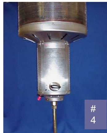
4. Remove the plastic protective end cap from only one end of the 3/8" male flared fitting at the end of the rigid fuel feed line. Leave the other end cap on to protect the fittings while you are proceeding with the assembly. Also remove the foam packing material on the fuel feed line. Either end of the fuel feed line can be attached to the heater head. **(See # 4)**
